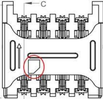
The diagram shows a cross-section of a SIM card connector assembly. It features a central SIM card slot with four pins on each side. A red circle highlights a new orientation mark on the metallic shell, which is a small square with a diagonal line. An arrow labeled 'C' points to the top of the shell, and another arrow points upwards from the shell.
